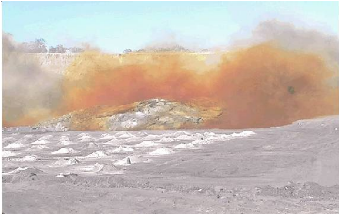
An example of blasting fume.
