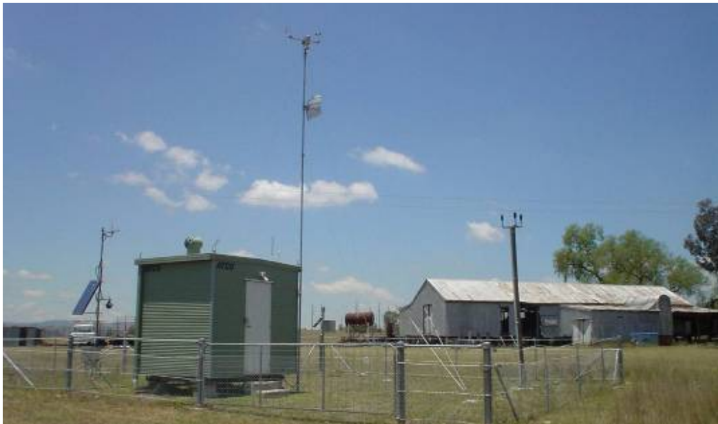
Example of Remote Monitoring set up including noise, weather and wireless comms
