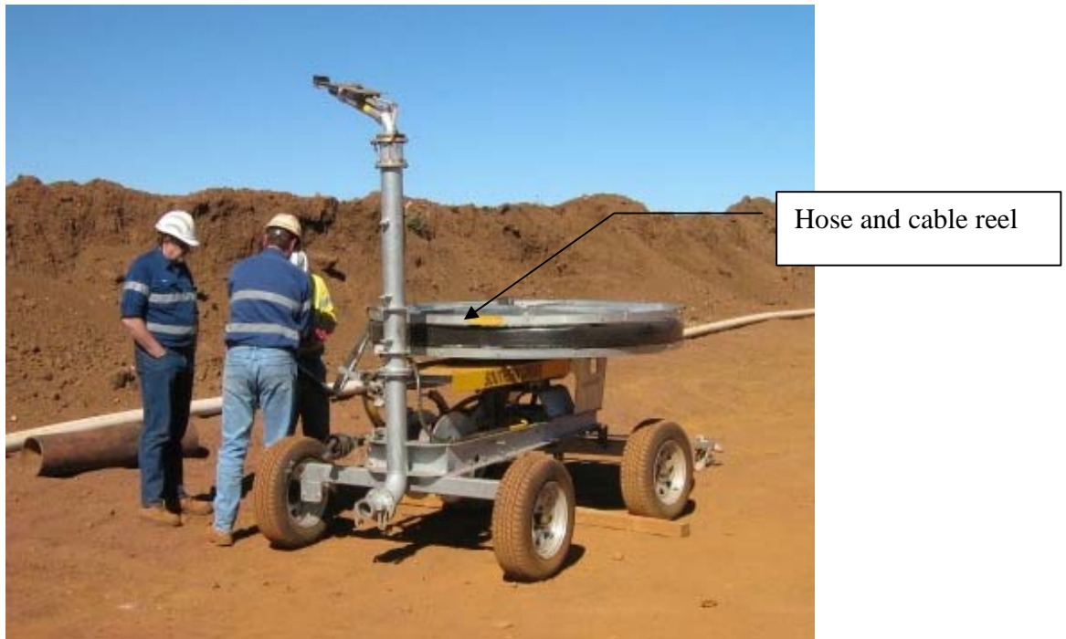
A typical mobile irrigator used on an iron ore mine
