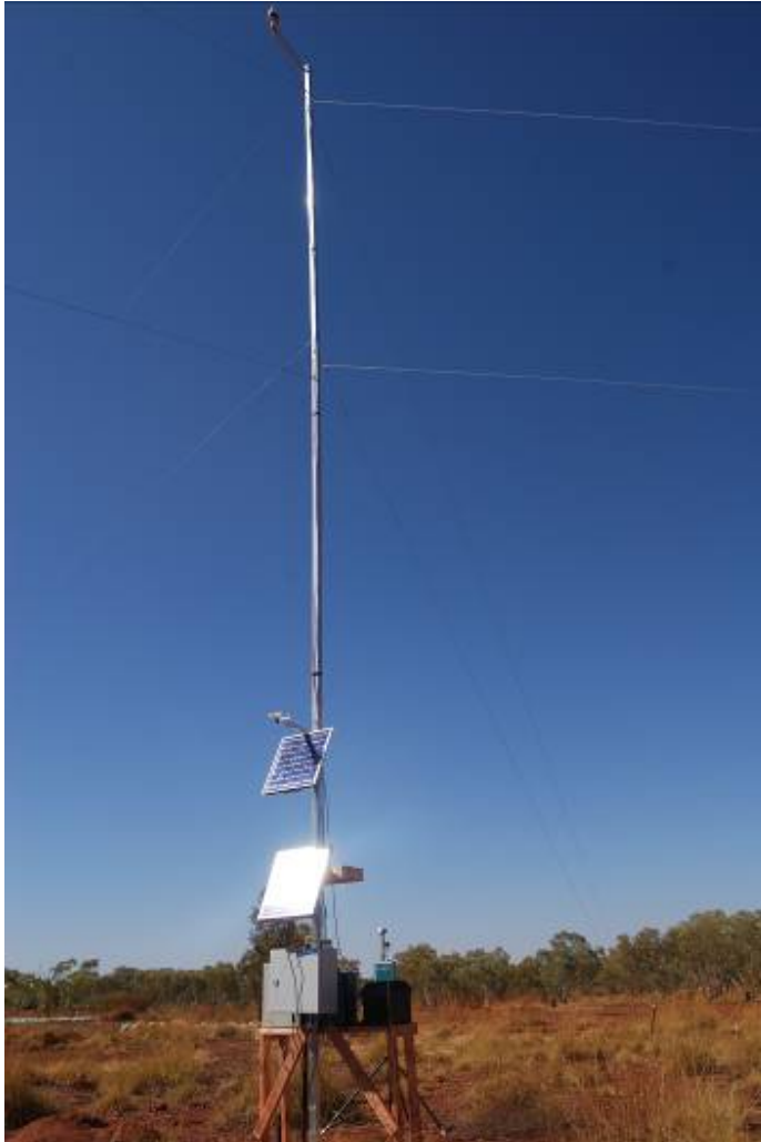
Weather station at a remote baseline monitoring site with solar power panels and low-power partisol dust monitor (right hand side of installation).
