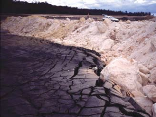
Batuan sisa didorong ke tailing kering
