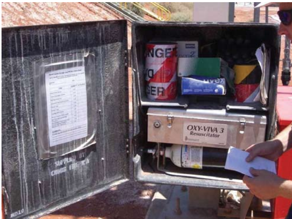
Cyanide Emergency Box
