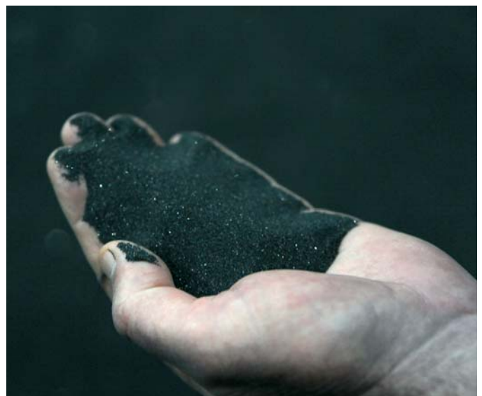
Synthetic rutile is a processed ilmenite with a composition of 88 to 95 percent titanium dioxide.
