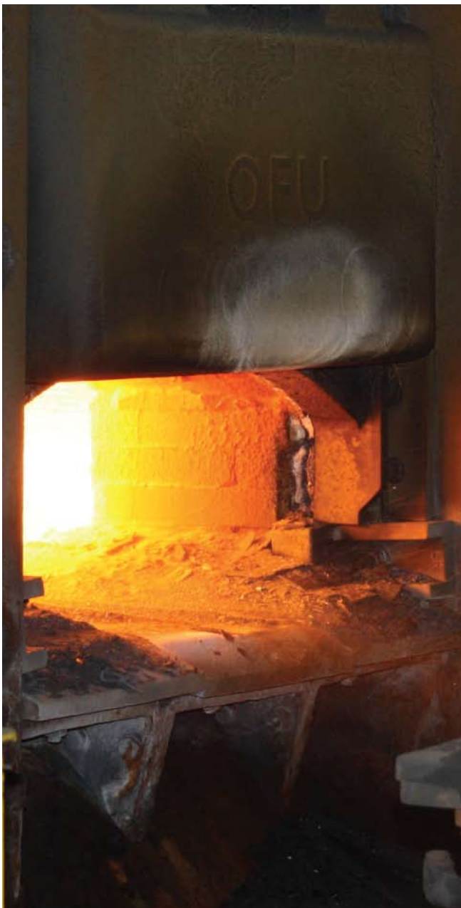
Steel billets are pushed from the reheat furnace
