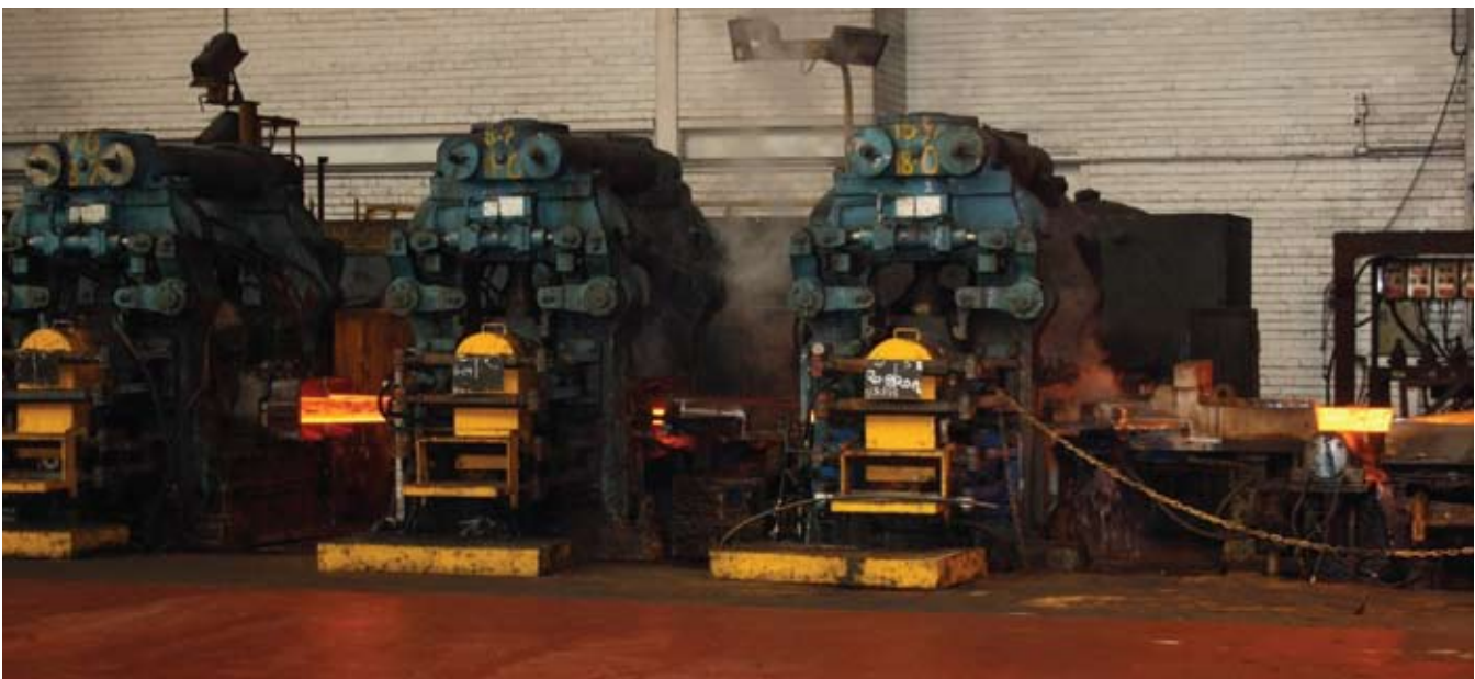
Billets travel through a series of rolling stands to change their size and shape
